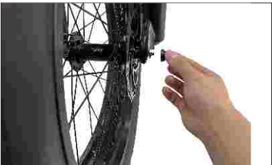
05 Insert the front wheel for quick release A: Adjust the screw pressure
