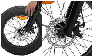
03 Remove the fork protector A: The protective shaft can be removed and thrown away
