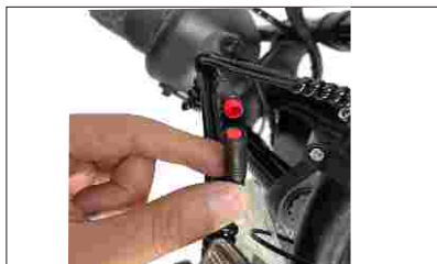
01 Waterproof line pull plug, pay attention to the good side of the mouth
