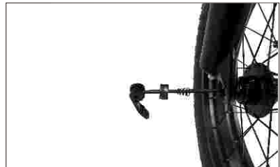
04 Put the wheel in the front fork Disc brake disc alignment clamp card slot
