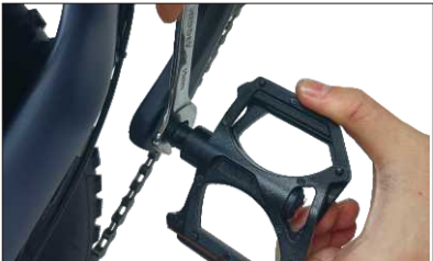
03 “R” pedal is fixed clockwise and fixed on the crank
