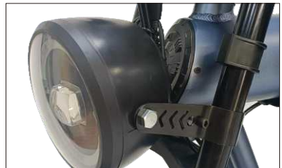
04 Fix the headlight on the fork as shown
