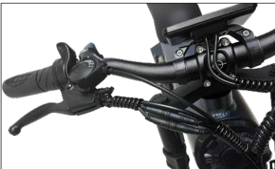
05 Connect the power-off brake handle waterproof cable
