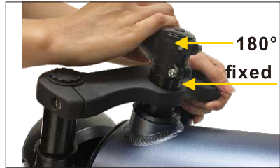
02 Fix the front shock absorber and rotate the riser 180°
