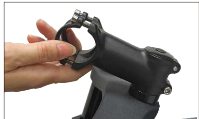
04 Remove front 4 bolts from stem cover then remove stem cover
