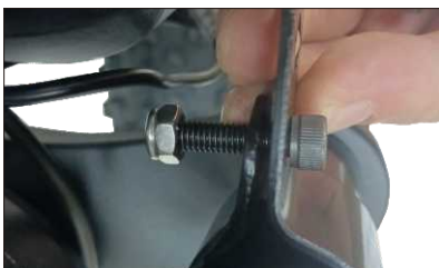
05 Remove taillight fixing screw
