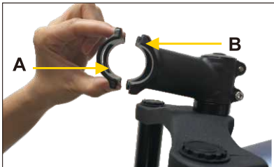
03 Tighten the side A, B screws
