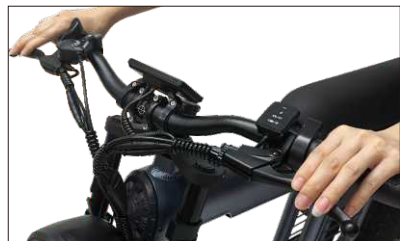
06 Adjust handlebar according to your needs , then ensure all bolts are tightened firmly
